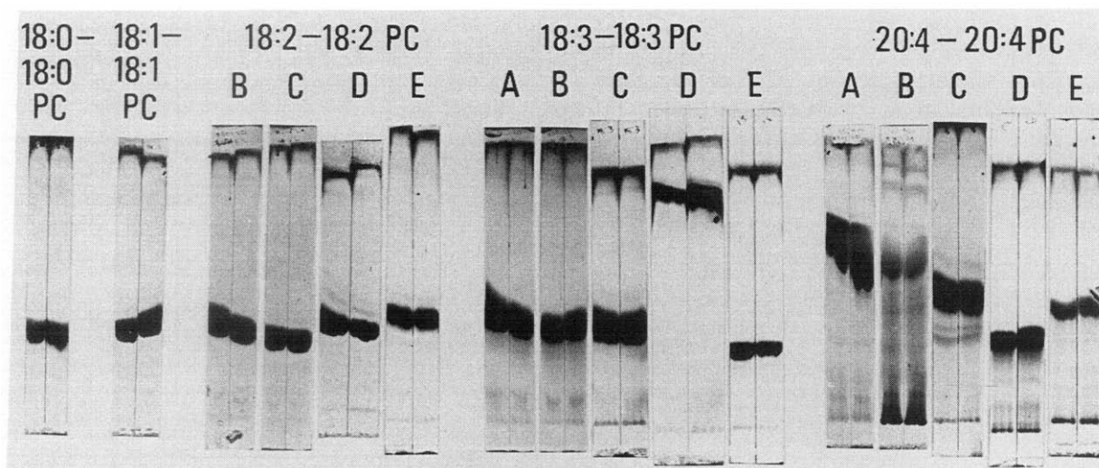
Fig. 2. Thin-layer chromatographic plates of the dipolyenoic phosphatidylcholines obtained after calorimetric analyses. This figure is a composite of lanes from chromatograms run at different times under different conditions of humidity and plate activation. The major spot of all samples had the mobility of PC as judged from the mobility of a PC standard in an adjacent lane. The labelling corresponds to that used in Table I.
